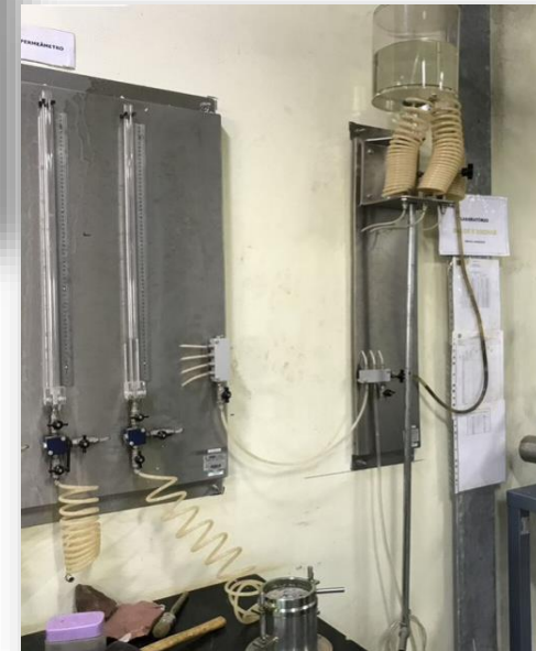
Fig. 9. constant load permeameter. Source: Carlos, 2021
