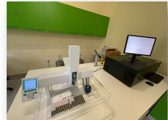
Fig. 11- Liquid Water Isotopic analyser. Source: Carlos, 2021
